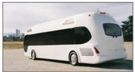
This three-foot model represents the fullsize, composite-bodied, hybrid fuel cell bus MES designed for the demonstration project.
