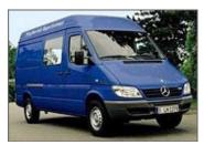
The Sprinter van is a prototype plug-in hybrid vehicle developed by EPRI and DaimlerChrysler.
