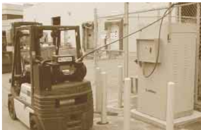
FuelMaker's refueling systems offer both time-fill and fast-fill refueling. Here a forklift refuels using the fast-fill method, allowing the driver to be back to work in 2 minutes with a full tank of CNG.
