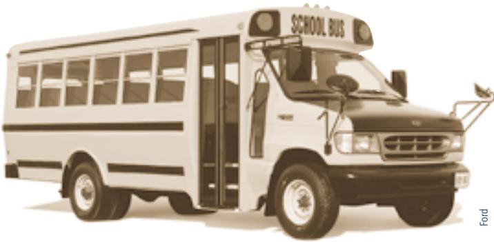
The E-450 Cutaway school bus has a 5.4-liter dedicated CNG V-8 engine and is expected to seat 30 students. It is rated as an ultra-low emission vehicle. According to Ford, using CNG reduces emissions of sulfur dioxide by 97 percent and carbon dioxide by 50 percent, compared with using gasoline. Emissions of particulate matter, a troublesome characteristic of diesel engines, are mostly eliminated with CNG.
