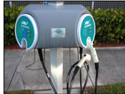
A Level-2 Charging Station (dual unit) with a standard cord set, carelessly stored by a user. This can create a tripping hazard, or allow rainwater to enter the connector – prematurely aging the equipment.
