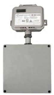
Con Edison's EV Load Measuring Device used as part of its Time of Use pilot.
