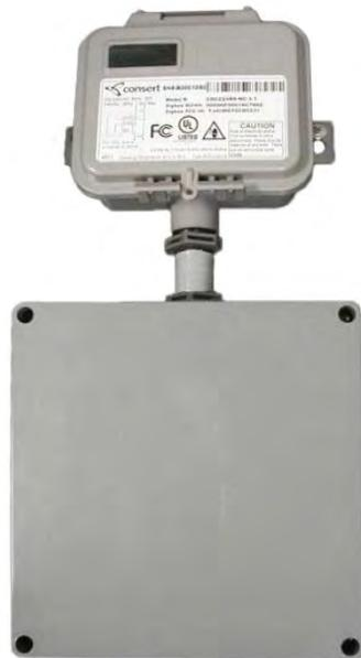
Con Edison's EV Load Measuring Device used as part of its Time of Use pilot.
