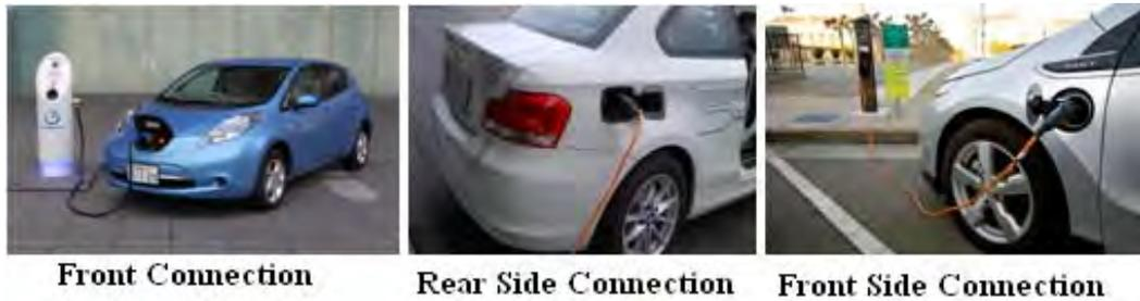
**Figure 12** Location of Charging Receptacle on an EV
