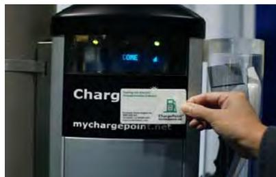
**Figure 17 RFID Card Example**
