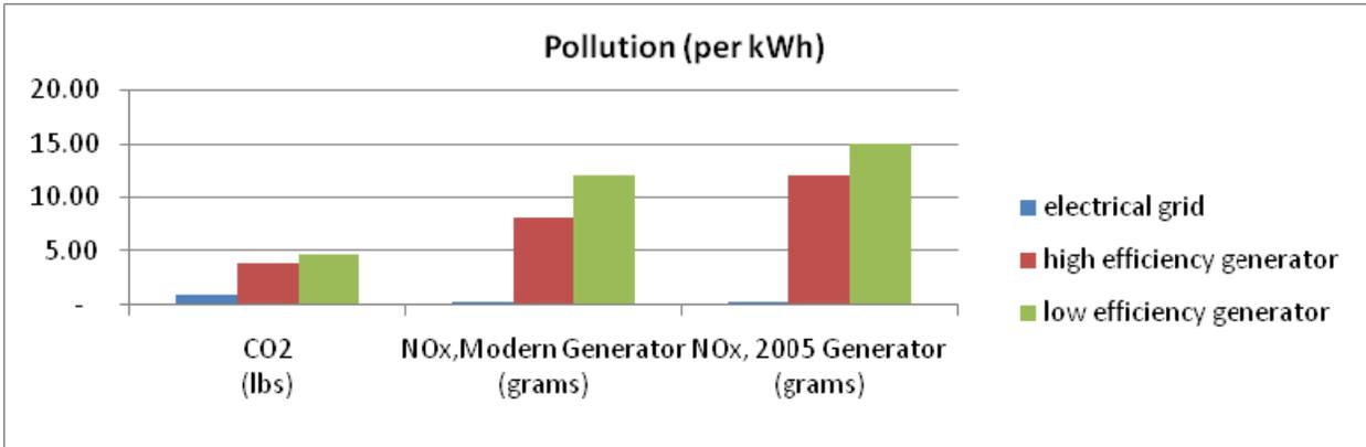
Figure 13: Pollution from Grid and Generator Power
