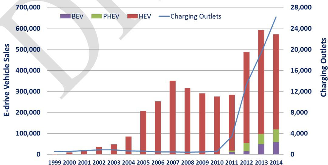
Fig. 4. Growth of annual sales of electric drive vehicles and plug-in charge points, 1999-2014
