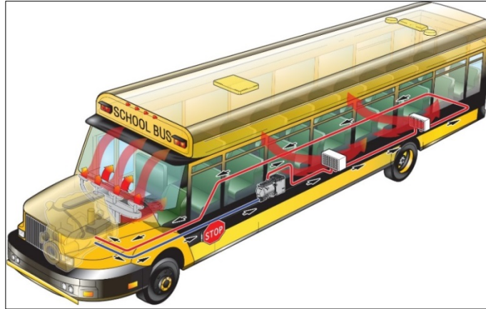
Figure 4.1. Heat distribution for school bus heater. (Image Courtesy of Espar Climate Systems)
