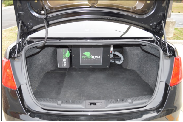
Figure 3.1. Police vehicle auxiliaries can be powered by a battery pack that fits in the vehicle's trunk. (Photo courtesy of ZeroRPM, Inc.)
