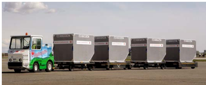
Air Canada with retrofit fuel cell baggage tug
