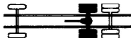
6x2 – 6 wheels, 2 driven 1 driving axle with tag axle
