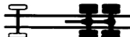
6x4 – 6 wheels, 4 driven 2 driving axles
