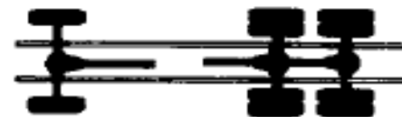
6x6 – 6 wheels, 6 driven 3 driving axles
