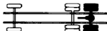
6x2 – 6 wheels, 2 driven 1 driving axle with pusher axle
