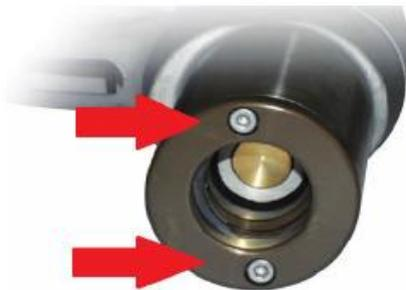
**IF A NOZZLE BECOMES DIFFICULT TO CONNECT OR DISCONNECT FROM A VEHICLE'S FILL PORT, LUBRICATION AND THIS SCREW TORQUE CHECK IS THE FIRST COURSE OF ACTION.**
