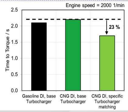
Engine full load performance with and without CNG DI optimized turbocharger and resulting time-to-torque comparison for Ford EcoBoost 1.0L engine using CNG DI system
