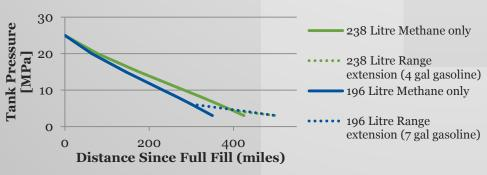
Illustration based on 26.5mpg, 75% gasoline usage in range extension, and 4 to 7 USgal gasoline tank. May need to limit 196 litre range to 450 miles due to Phase 2 EPA/NHTSA rules.
