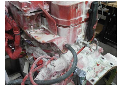
Photo of SLT2 Engine 'Post Test' (note the scale formation due to water spray)
