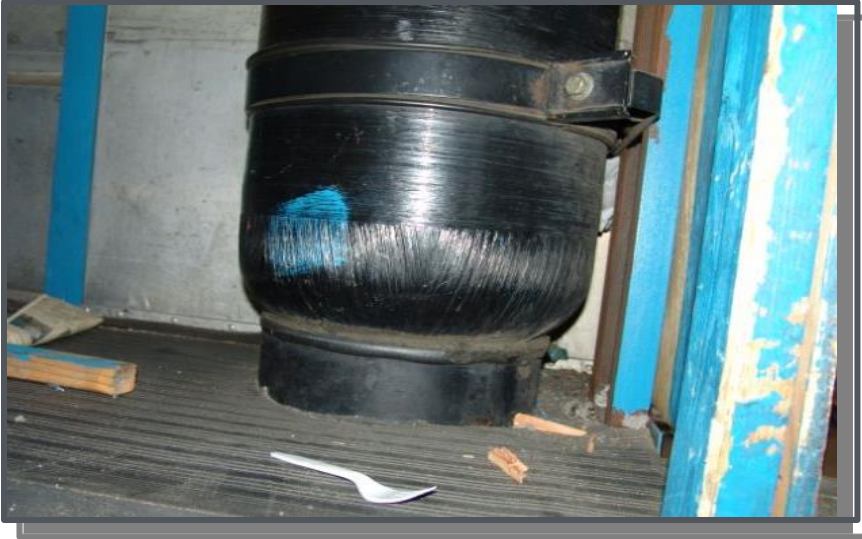
Cylinder improperly mounted on steel ring
