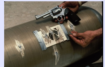
CNG Cylinder Severe Abuse Test 1983
