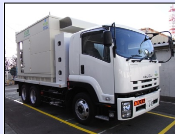
Tokyo Gas compressor truck
