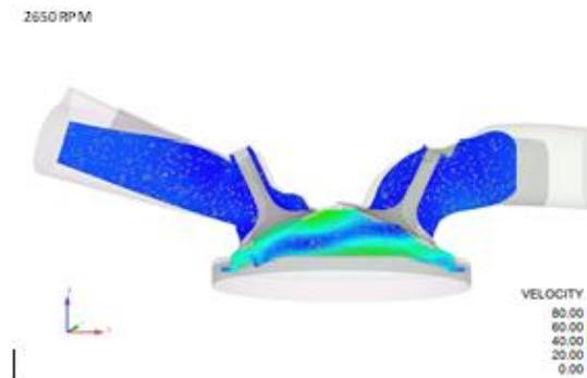
VELOCITY CONTOUR AT SPARK TIMING
