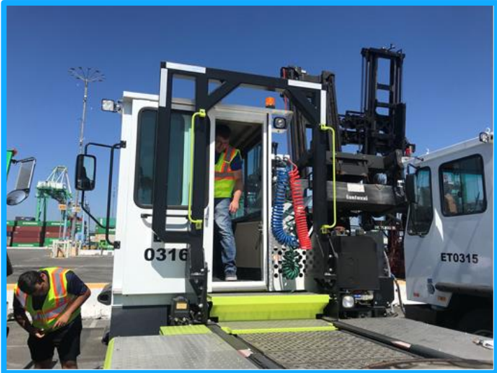
August 20: Inspecting BYD battery-electric tractor for data port to install PAMS
