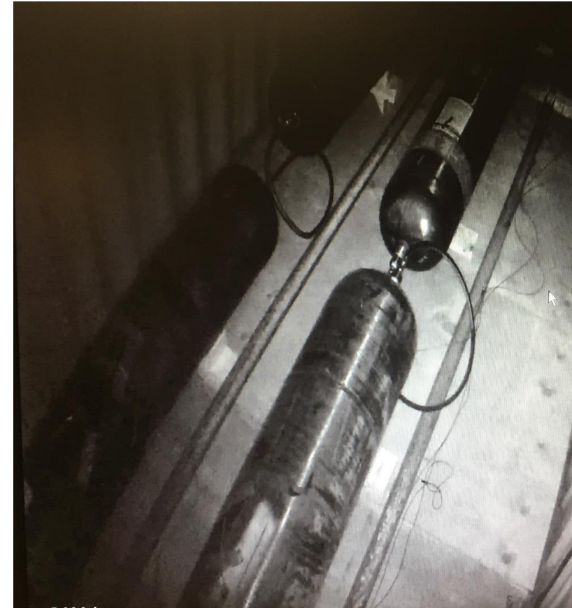
Four (4) tanks being simultaneously fatigue cycled tested
