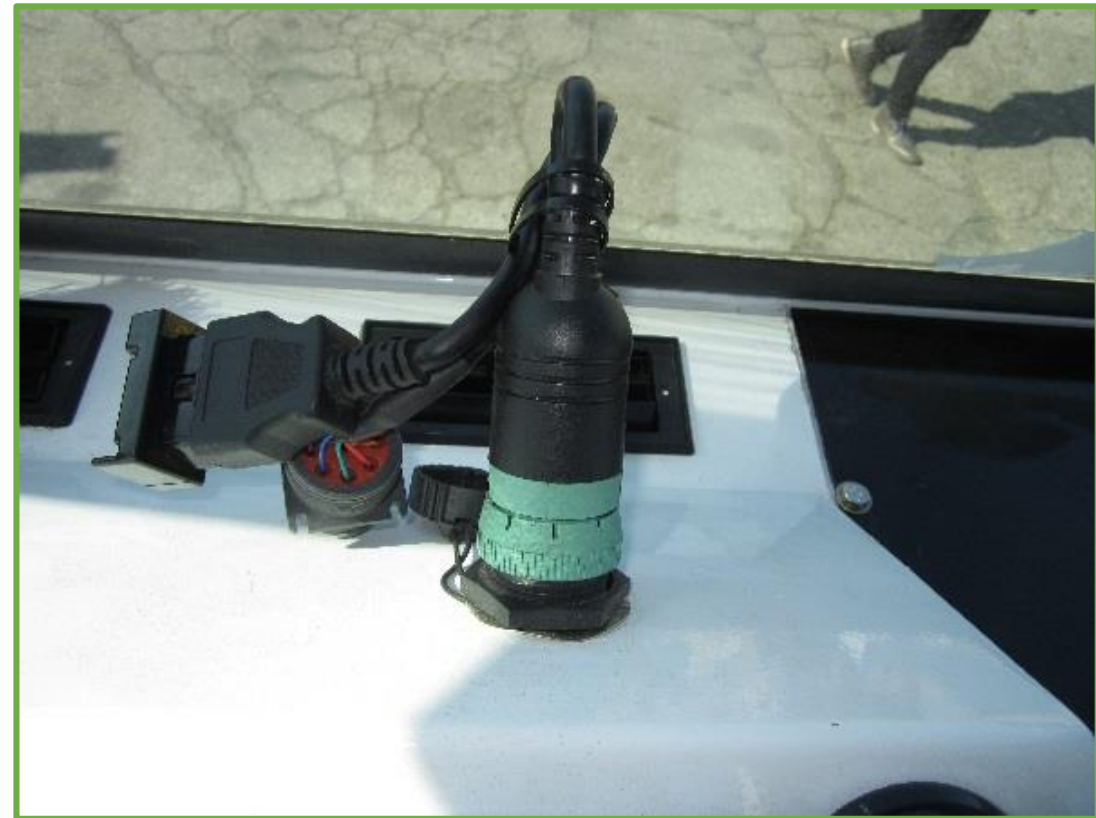
PAMS installed in J1939 port of Unit #483 LNG yard tractor
