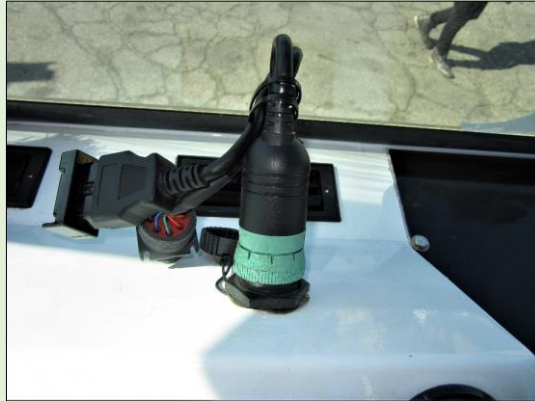
Trucks get Portable Activity Monitoring Systems (PAMS) installed; PAMS device plugged into the LNG UTR's J1939 port
