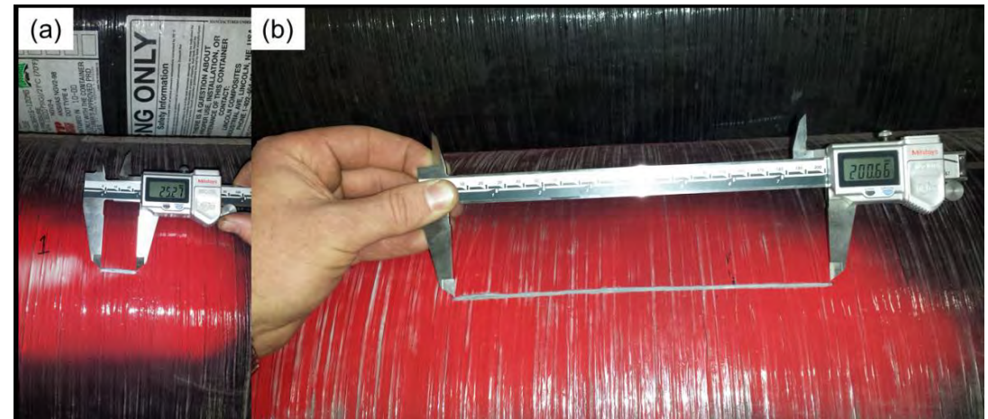
(a) short width, deeper depth notch and (b) longer width, shallower depth notch
