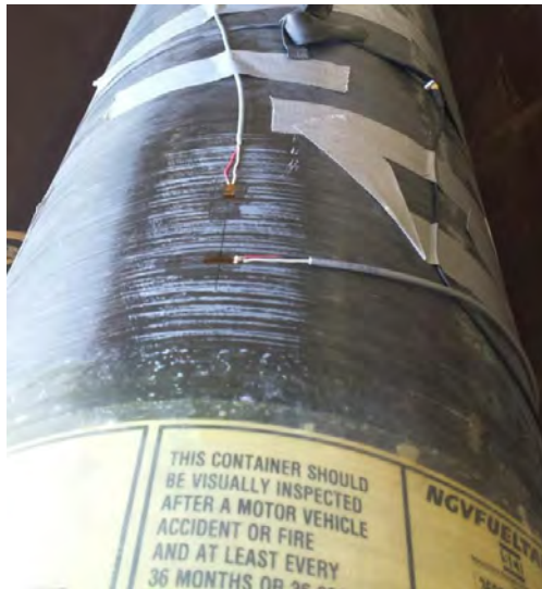
Axial and hoop oriented strain gages for burst testing
