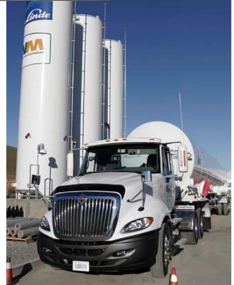
Most of the vehicles that use RNG in the U.S. are refuse trucks. At California's Altamont Landfill, tankers fill up with liquefied RNG and distribute it for use in 350 refuse trucks throughout the state. *Photos from Waste Management*
