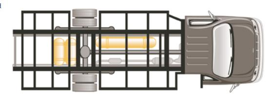
Ford's CNG-fueled E-450 Cutaway has one underbody mid-ship fuel tank and two aft-axle tanks. Fuel capacity is 16.7 gasoline gallons equivalent.
