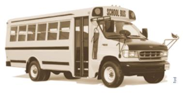
The E-450 Cutaway school bus has a 5.4-liter dedicated CNG V-8 engine and is expected to seat 30 students. It is rated as an ultra-low emission vehicle. According to Ford, using CNG reduces emissions of sulfur dioxide by 97 percent and carbon dioxide by 50 percent, compared with using gasoline. Emissions of particulate matter, a troublesome characteristic of diesel engines, are mostly eliminated with CNG.
