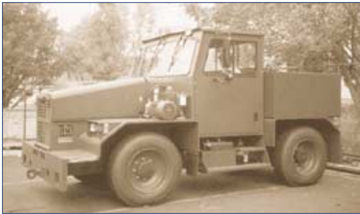
Hybrid-electric tow tractors at Robins mate a Cummins diesel engine with 48 lead-acid batteries and a 100-kilowatt Seimens motor.
