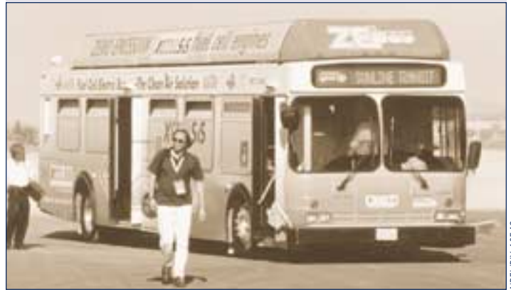
The ZEBus, operated by SunLine Transit, demonstrated superior range due to roof-mounted hydrogen fuel supplies.
