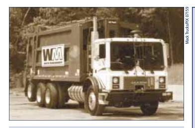
This refuse hauler, operated by Waste Management in Washington, Pennsylvania, runs on a Mack E7 natural gas (LNG) engine.
