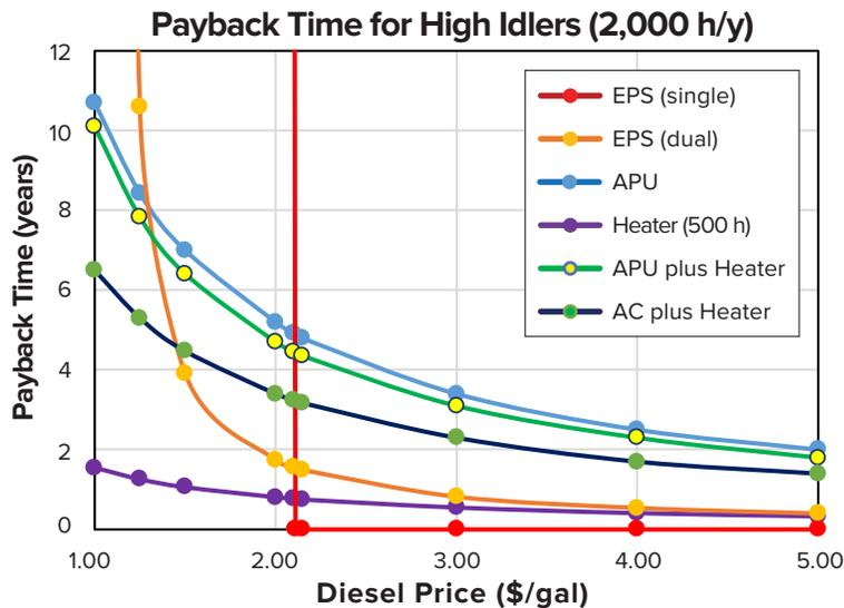
Figure 1. Equipment payback time as a function of fuel price for high idlers (2,000 h/yr). (Assumptions: idling fuel consumption = 0.8 gal/h; EPS cost, single system = \$1.85/h; EPS cost, dual system = \$1.00/h.)
